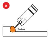
Unstable arc, spatter, poor penetration and fusion.
