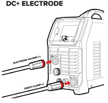
For DCEN electrodes, connect the earth clamp to the
