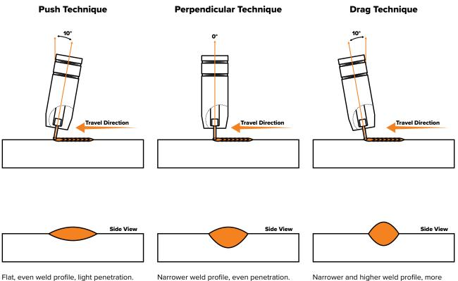
Narrower weld profile, even penetration.
