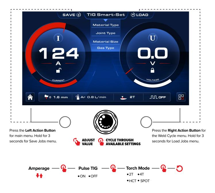
*Note:* The adjustable settings can be limited by the specifications chosen in the setup wizard.
