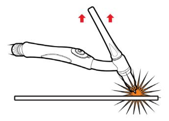
**18.** If you have the machine setup in 4T mode, you can release the trigger after initiating the arc. To end the weld press the trigger again and hold the torch there for the length of the post gas.
