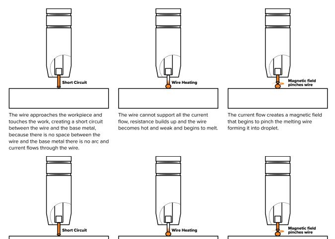
The pinch causes the forming droplet to separate and fall towards the forming weld pool.
