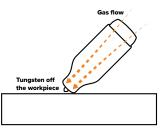
Lay the nozzle on the job without the tungsten touching the work.
