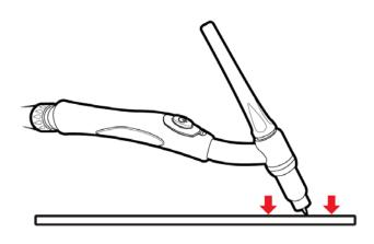
**17.** If you have the machine setup in 2T mode, you will need to hold the trigger for the remainder of the weld. To end the weld, let go of the trigger and hold the torch there for the length of the post gas to ensure the weld has gas coverage while cooling.
