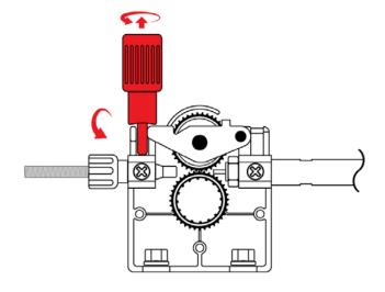
**4.** You now have access to the drive roller. When reinstalling, ensure you line up the key slot.
