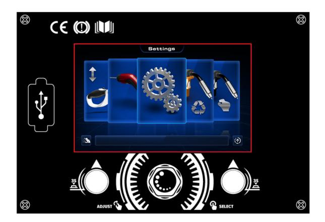
Navigate to the settings menu by using the scroll knob. Enter the menu by pressing the scroll knob down.
