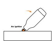
Rock the torch back in the opposite direction, the arc will ignite as the tungsten lifts off the work.
