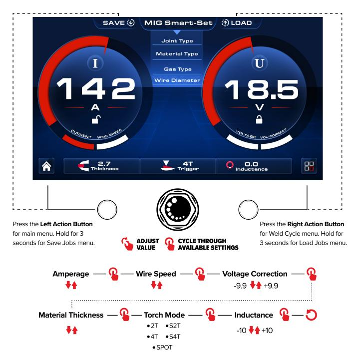
*Note:* The adjustable settings can be limited by the specifications chosen in the setup wizard.
