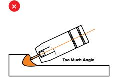
Poor control, unstable arc, less penetration, lots of spatter.
