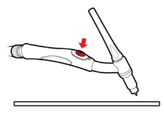
**14.** For Lift TIG, begin with the tungsten off the workpiece, Press the button on the torch to initiate the gas flow.
