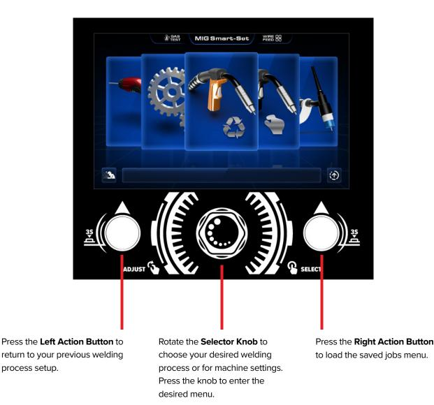
**Note:** While hovering over MIG Smart-Set Mode or MIG Manual mode, you can perform a gas test by pressing and holding the **Left Action Button.** You can also feed wire by pressing and holding the **Right Action Button.**
