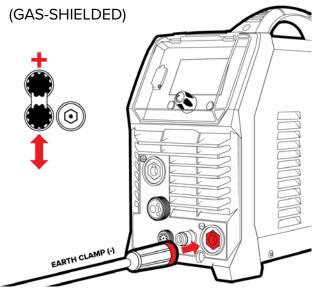
With the polarity connectors and the earth clamp installed into the correct dinse ports for the polarity you wish to run, now install the MIG torch into the Euro Connect Port. Ensure you line up the internal ports correctly. 6. For DCEN (-) start by putting the polarity connector to negative. Inside the machine loosen the polarity connector knobs, and orientate the polarity bar horizontally, then re-tighten the knobs. Twist the earth clamp into the positive (+) dinse port.
