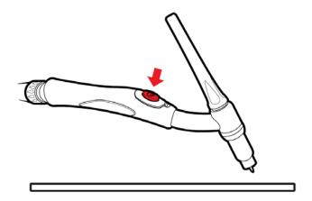
**15.** Gently touch the tip of the tungsten to the workpiece.
