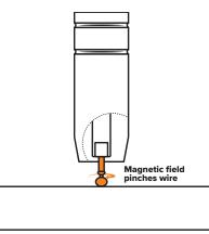
The wire feed speed overcomes the heat of the arc and the wire again approaches the work to short circuit and repeat the cycle.
