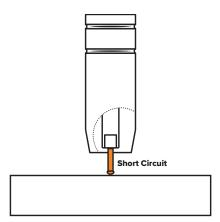
The wire approaches the workpiece and touches the work, creating a short circuit between the wire and the base metal, because there is no space between the wire and the base metal there is no arc and current flows through the wire.
