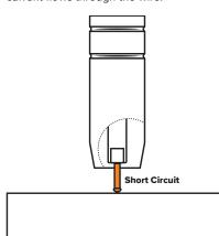
The pinch causes the forming droplet to separate and fall towards the forming weld pool.
