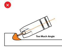
Poor control, unstable arc, less penetration, lots of spatter.
