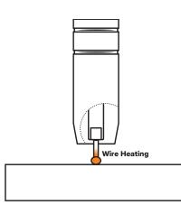
An arc is created at the separation of the droplet and the heat and force of the arc flattens out the droplet into the weld pool. The heat of the arc melts the end of the wire slightly as it feeds towards the base metal.
