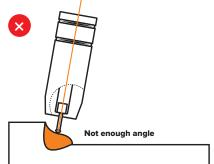
Less control over the weld pool, more spatter.
