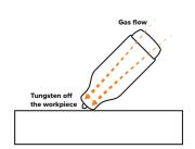
Lay the nozzle on the job without the tungsten touching the work.
