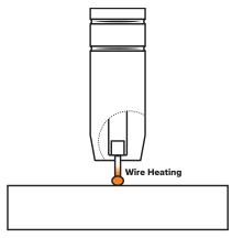
The wire cannot support all the current flow, resistance builds up and the wire becomes hot and weak and begins to melt.
