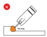
Unstable arc, spatter, poor penetration and fusion.
