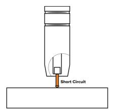
The pinch causes the forming droplet to separate and fall towards the forming weld pool.
