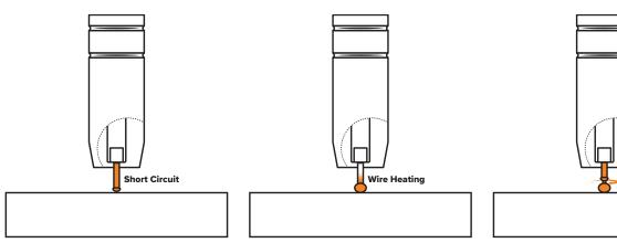
The wire approaches the workpiece and touches the work, creating a short circuit between the wire and the base metal, because there is no space between the wire and the base metal there is no arc and current flows through the wire. The wire cannot support all the current flow, resistance builds up and the wire becomes hot and weak and begins to melt. The current flow creates a magnetic field that begins to pinch the melting wire forming it into droplet.
