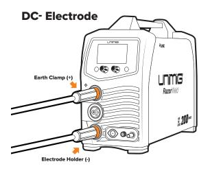
Connect the plug into a 15 AMP socket, then switch the machine ON.
