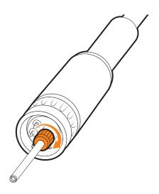
Loosen the inlet guide tube retaining screw.
