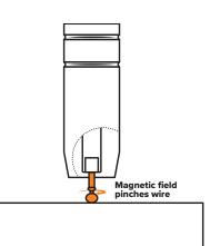
The wire feed speed overcomes the heat of the arc and the wire again approaches the work to short circuit and repeat the cycle.
