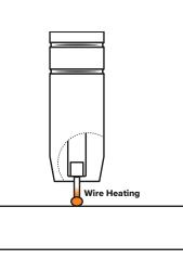
An arc is created at the separation of the droplet and the heat and force of the arc flattens out the droplet into the weld pool. The heat of the arc melts the end of the wire slightly as it feeds towards the base metal.
