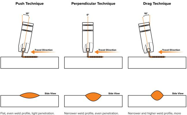
Narrower and higher weld profile, more penetration.
