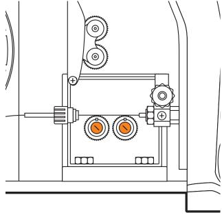
Ensure you have V Groove drive rollers installed. If not, fit correct rollers and replace the roller covers.
