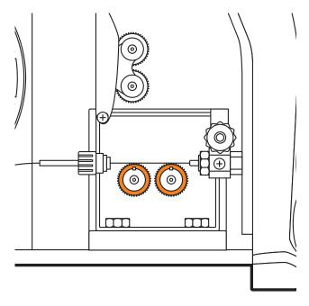
Take the extended aluminium liner all the way up and over the drive roller.
