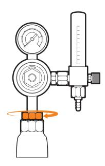
Connect gas hose to the flowmeter outlet, and 8 Adjust gas flow to 6-10L/min. crimp in place.
