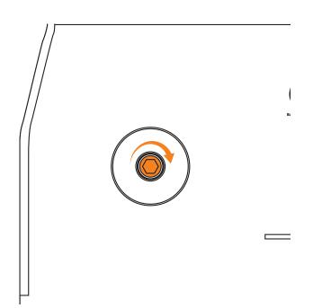
1 Connect the polarity connector to the **positive (+)** connection, unscrew the bolt and move the connector then screw and tighten in place.
