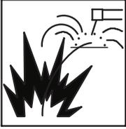
**Fire hazard.** Welding/cutting on closed containers, such as tanks, drums, or pipes, can cause them to explode. Flying sparks from the welding/cutting arc, hot workpiece, and hot equipment can cause fires and burns. Accidental contact of the electrode to metal objects can cause sparks, explosion, overheating, or fire. Check and be sure the area is safe before doing any welding/cutting.
