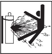
**Gas Cylinders.** Shielding gas cylinders contain gas under high pressure. If damaged, a cylinder can explode. Because gas cylinders usually are part of the welding/cutting process, be sure to treat them carefully. CYLINDERS can explode if damaged.
