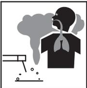
**Fumes and gases are dangerous.** Smoke and gas generated while welding or cutting can be harmful to people's health. Welding produces fumes and gases. Breathing these fumes and gases can be hazardous to your health.
