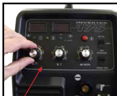
(6) Set the welding current using the amperage control dial
