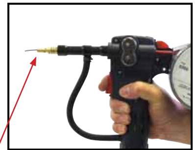
(10) Remove the gas nozzle and contact tip. Pull the trigger to drive the wire through the neck until it exits the contact tip holder
