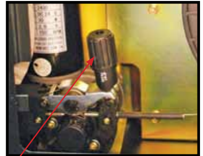
(10) Apply a medium amount of pressure to the drive roller
