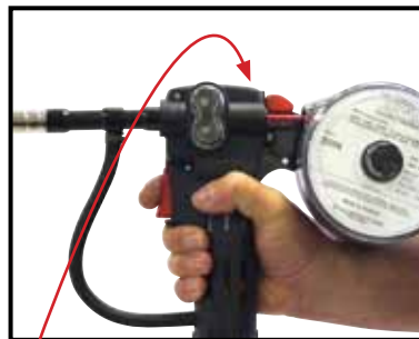
(12) Adjust the drive roll pressure if required by using the adjusting screw at the top of the torch.
