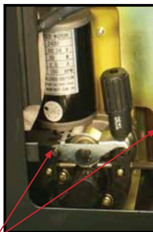
(6) Fit the correct sized Knurled Drive roller for Gas Less Flux Cored wire
