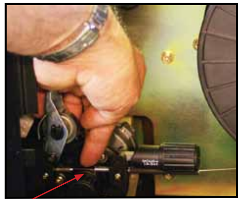
(8) Feed wire over the drive roller into the outlet guide tube, Push the wire through approx 150mm.
