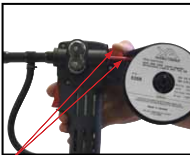
(8) Carefully feed the wire through the inlet guide tube onto the drive roller through into the outlet guide tube. Push down the tension arm lever to release the pressure of the drive roller allowing the wire to be guided through the drive roller into the gun neck.
