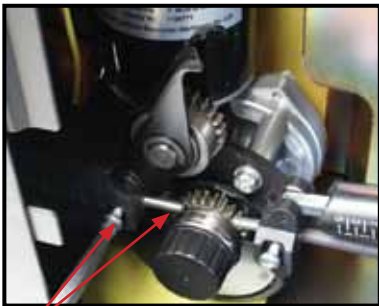
(10) Loosen the inlet guide tube retaining screw.
