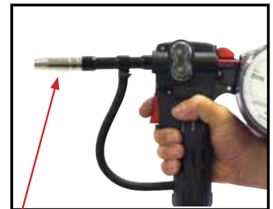
(13) Fit the gas nozzle ready for welding.
