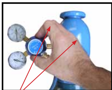
(5) Carefully open the valve of the gas cylinder, set the flow to 6-10 l/min
