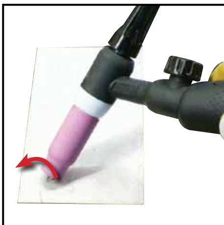
(8) With a small movement rotate the Gas Cup forward so that the Tungsten Electrode touches the work piece.
