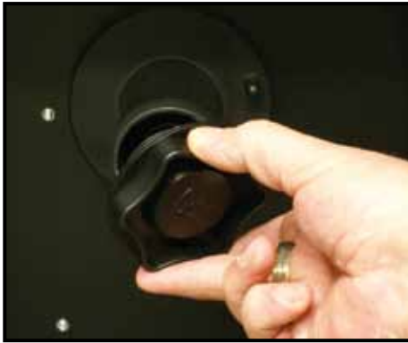
(1) Remove the spool retaining nut.
