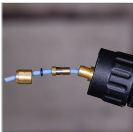
(7) Fit the liner collet, liner O-ring and liner retaining nut.
