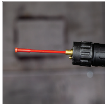
(3) Carefully pull out and completely remove the liner
