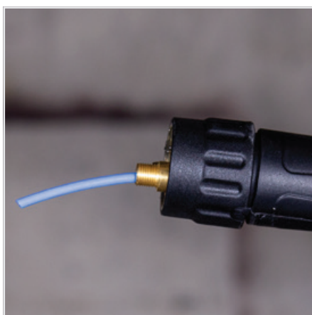
(5) Carefully feed in the new liner in short forward movements down the torch lead all the way to exit the torch neck. Be careful not to kink the liner
