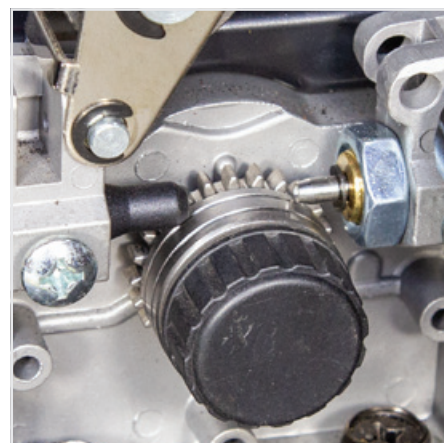
(9) Install a U groove drive roller of the correct size for the diameter wire being used.
