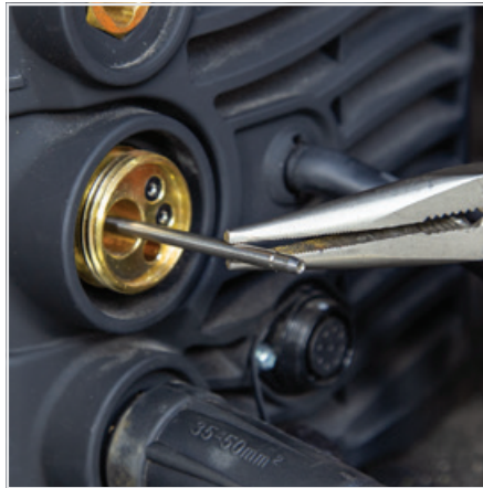
(11) Remove the inlet guide tube using long nose pliers.
