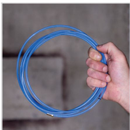
(4) Carefully unravel the new liner
