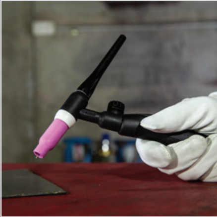
(1) Assemble front end parts of the TIG torch, fitting a sharpened tungsten suitable for DC welding.
