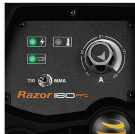
(7) Set the welding current using the amperage control dial.
